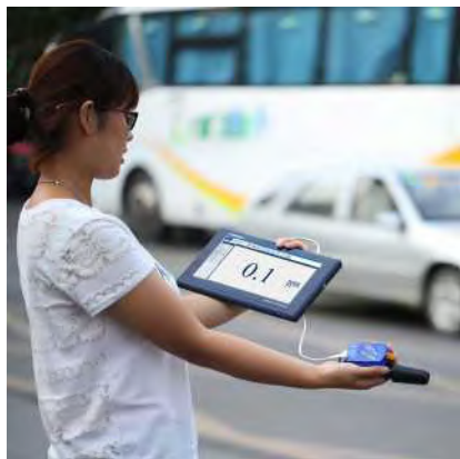
Experiment of testing of NO 2 content in vehicle exhaust with Ilongwill® NO 2 sensor and Ilongwill® digital display module
