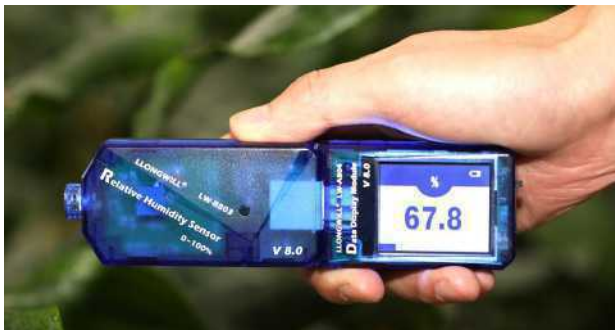
Relative humidity sensor is connected to Sensor Data Display Module
