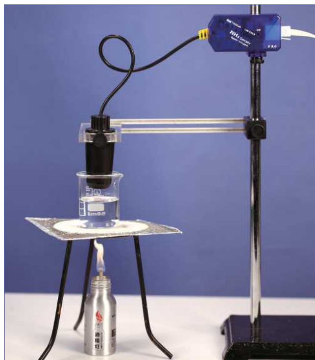
Detection of NH_4^+ with NH_3 sensor
