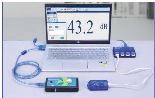
An automatic control system composed of Pad terminal, actuator and sound level sensor
