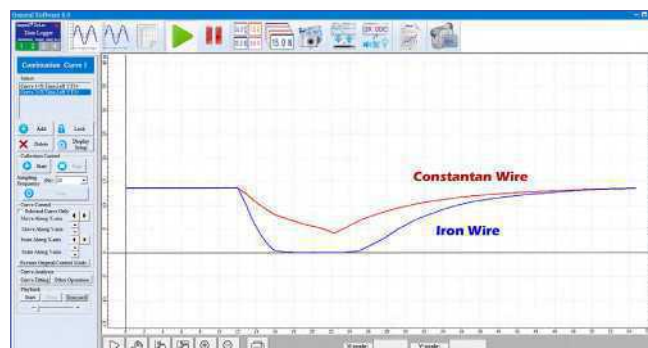
The force curve declined during the wire being heated. It demonstrates the wire's expansion.
