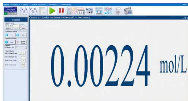
Experiment results of \text{Cl}^- content in table salt.
