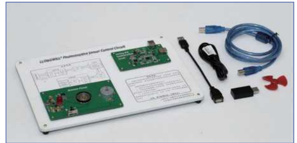
Photosensitive sensor control circuit
