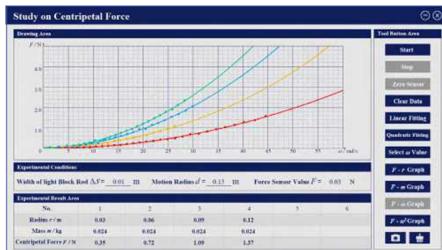
Curve of relationship between centripetal force F and angular velocity \omega
