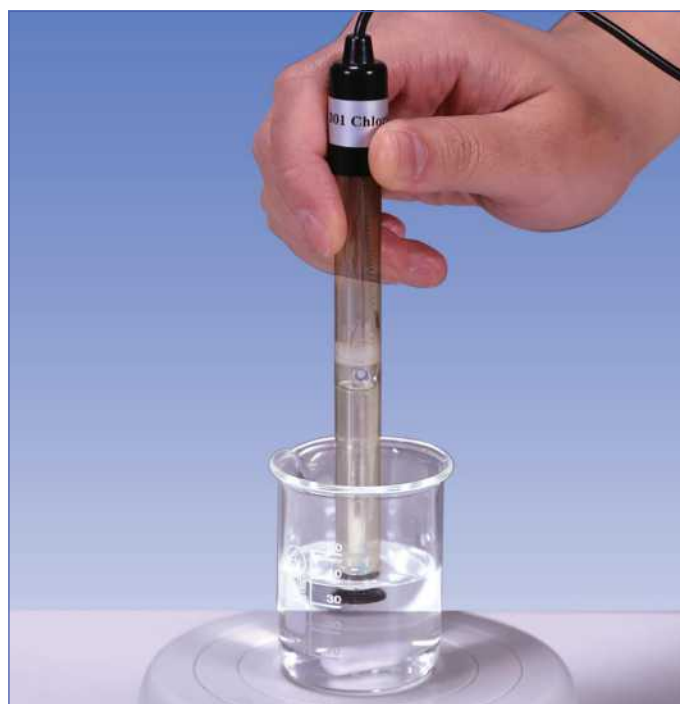
Experiment of \text{Cl}^- content in table salt by using chloride ion sensor
