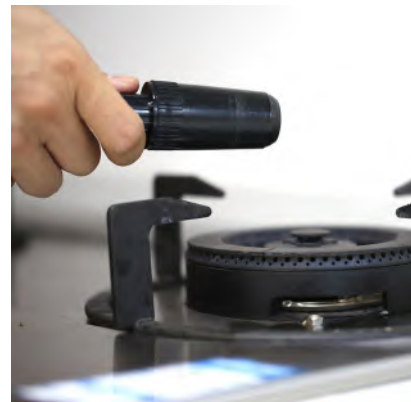
Detection of gas composition by using CH 4 sensor
