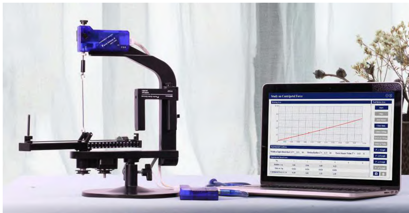
Experiment fitting curve ( F-m ) between the centripetal force and the mass
