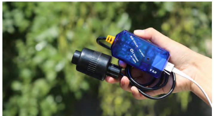
Measuring O 2 content in forest with O 2 sensor
