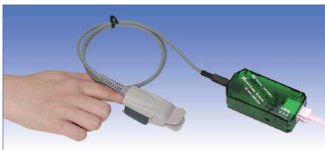
To measure the heart rate using sensor
