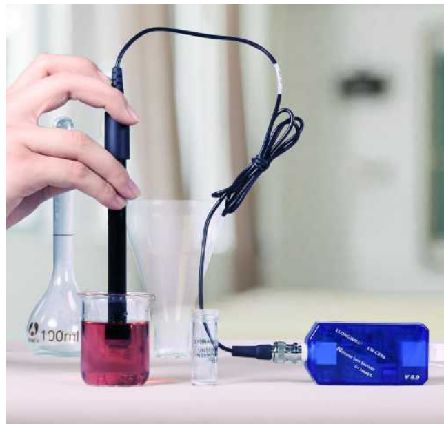
Determination of \text{NO}_3^- concentration in the fruit juice
