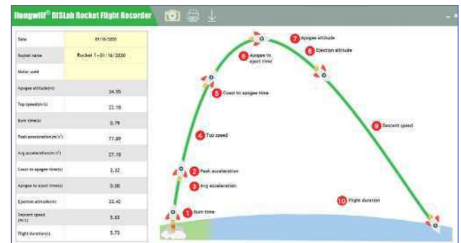
Data recording of rocket flight recorder during flight
