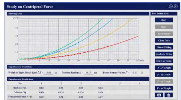
Experiment results of the relationship between the centripetal force F and angular velocity \omega
