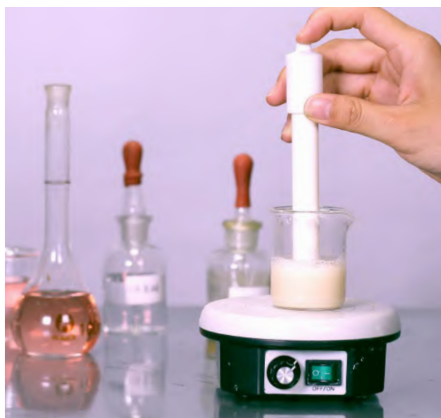
The experiment of study on the respiration of saccharomycetes by using CO 2 Sensor (Dissolved)
