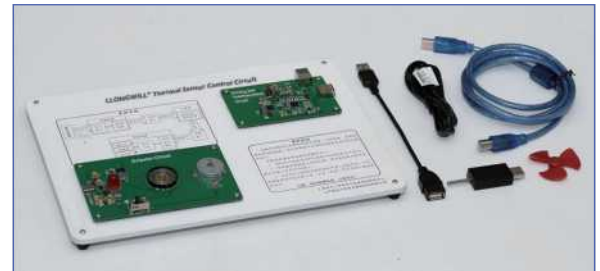
Thermal sensor control circuit
