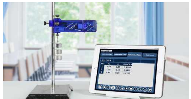
Gravity-mass relationship experiment (above) and experiment results(below)
