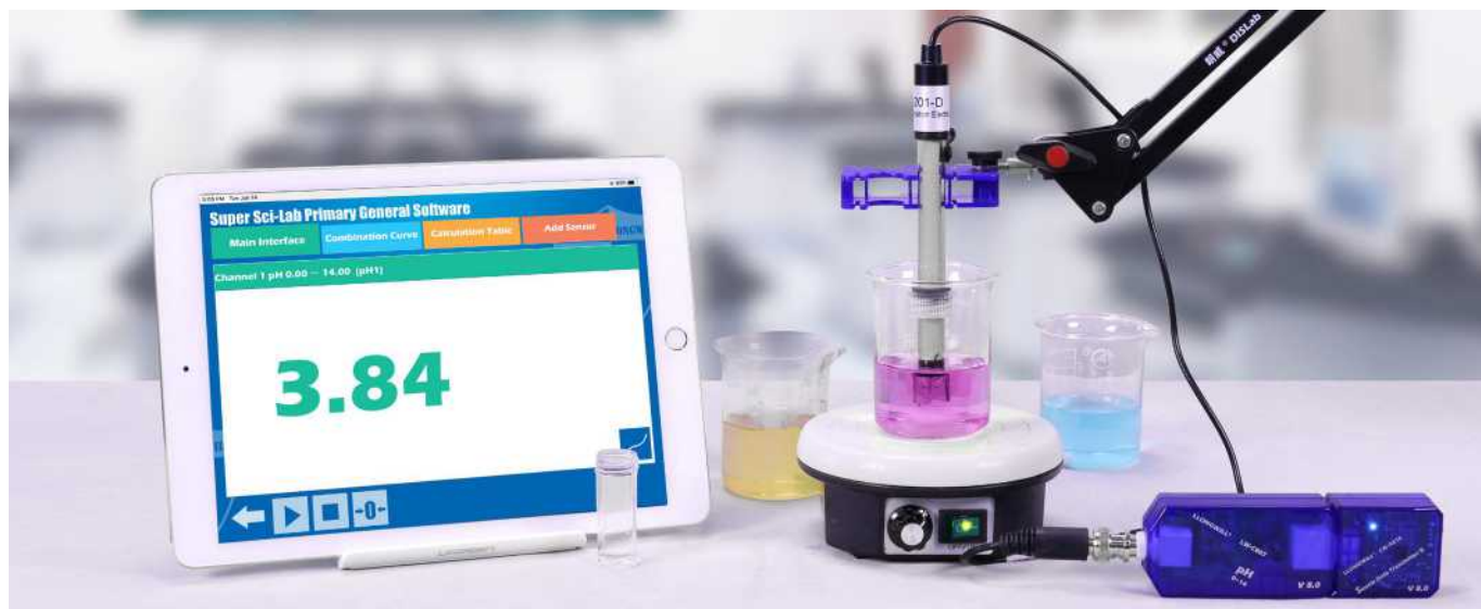
Measure the pH value of fruit juice by using pH sensor
