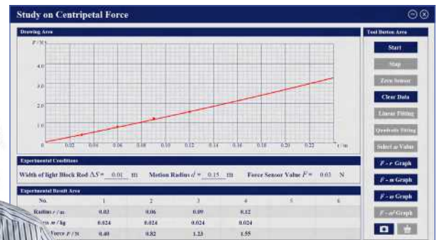
Experiment fitting curve ( F-r ) on the centripetal force and radius
