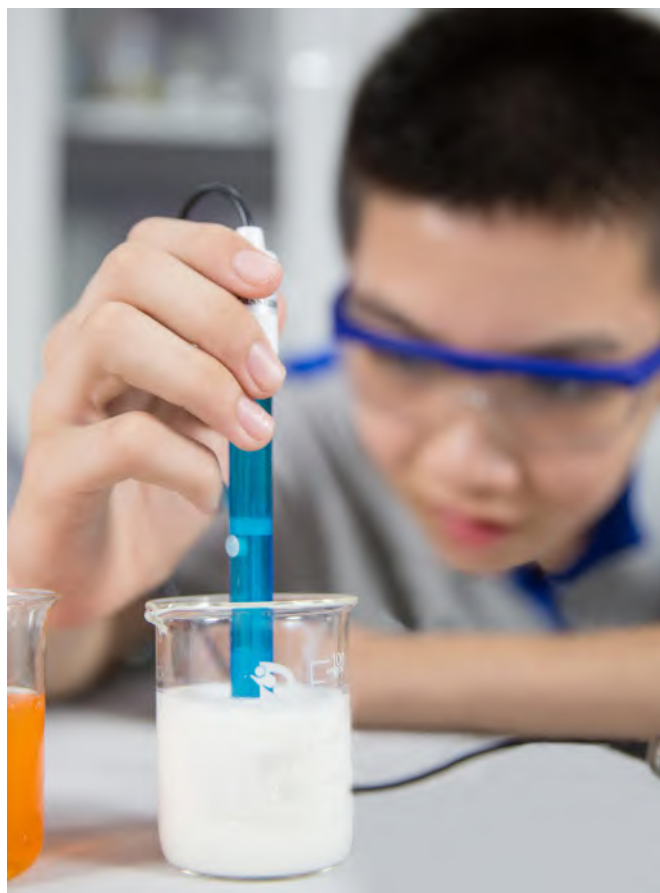
Concentration determination of NH 4 + in chemical fertilizer
