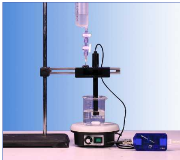
Use \text{CH}_3\text{COOH} solution to titrate with \text{NH}_3\cdot\text{H}_2\text{O} solution
