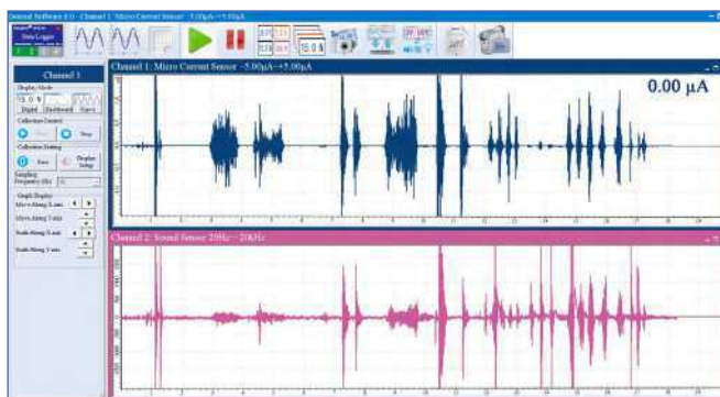
Waveform and sound of current at the receiving end
