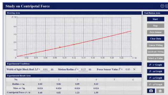
Experiment fitting curve ( F-m ) between the centripetal force and the mass
