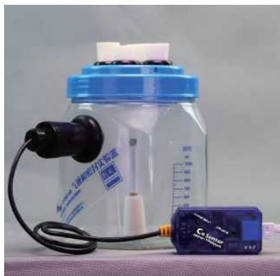
Experiment of CO content generated during cigarette combustion measured by using Ilongwill® CO sensor
