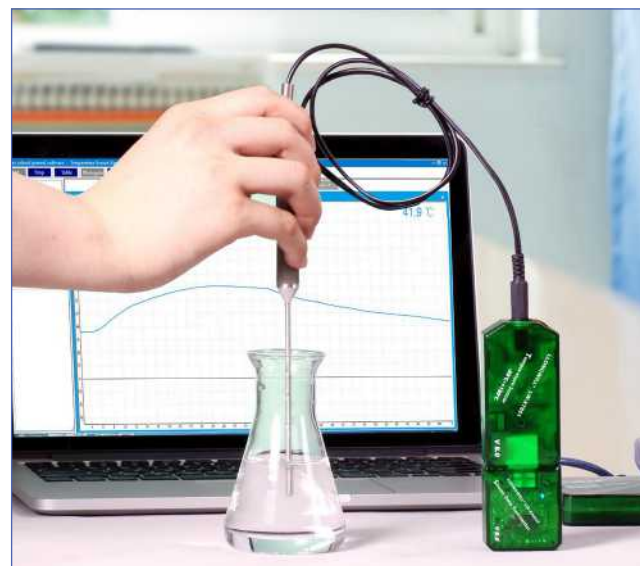
Temperature change during water cooling
