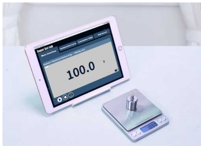
Wireless data reading of online electronic balance
